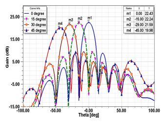
Fig. 6. Beam steering of 8x8 ESPAA
