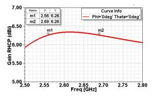
Fig. 3. Peak gain of antenna over the frequency band
