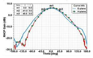
Fig. 9 (a). Measured radiation pattern at 2.57 GHz
