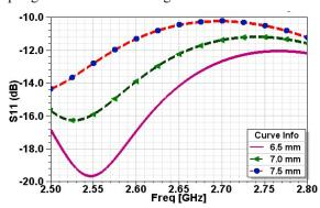
Fig. 4(a). Effect of cavity height on reflection coefficient
