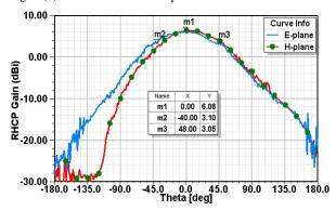
Fig. 9 (b). Measured radiation pattern at 2.69 GHz
