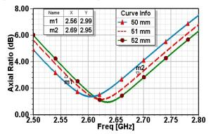
Fig. 4(c). Effect of cavity size on axial ratio
