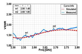
Fig. 8 (a). Simulated and measured VSWR plot
