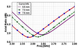
Fig. 4(b). Effect of cavity height on axial ratio
