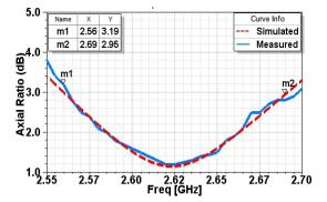
Fig. 8 (b). Simulated and measured axial ratio plot
