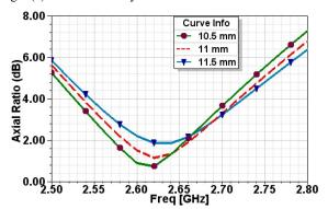
Fig. 4(d) Effect of the size of truncation on axial ratio
