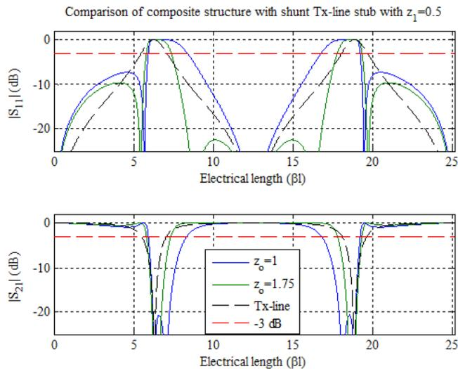
Fig.6 S-parameters comparison with Tx-line stub. Tx-line stub impedance is 0.5.
