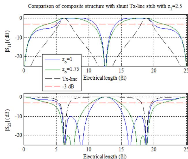
Fig.8 S-parameters comparison with Tx-line stub. Tx-line stub impedance is 2.5.
