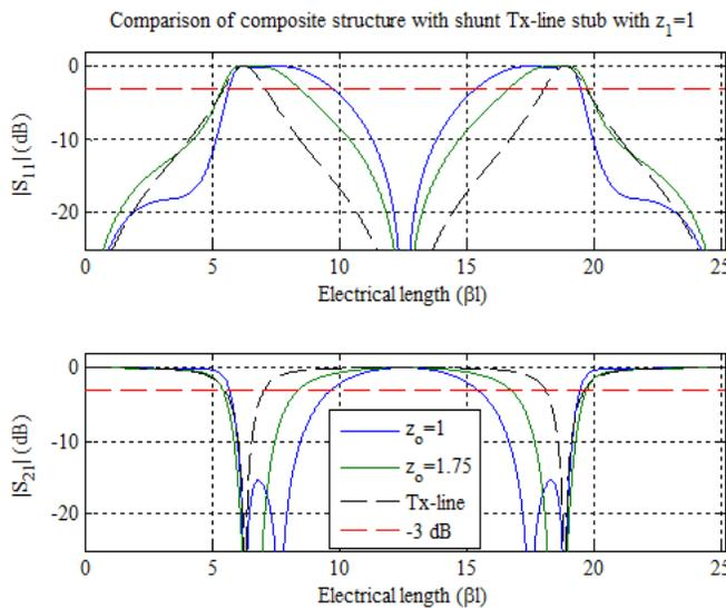
Fig.7 S-parameters comparison with Tx-line stub. Tx-line stub impedance is 2.5.
