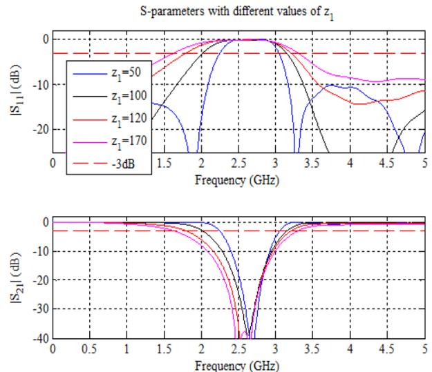
Fig.12 Full-wave simulations of AS-PCL for different -Tx line impedances.
