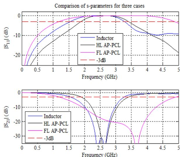
Fig.11 Full wave simulations of all-stop PCL +Tx line, all-stop PCL (HL) +all-pass PCL, and all-stop PCL(FL)+all-pass PCL.
