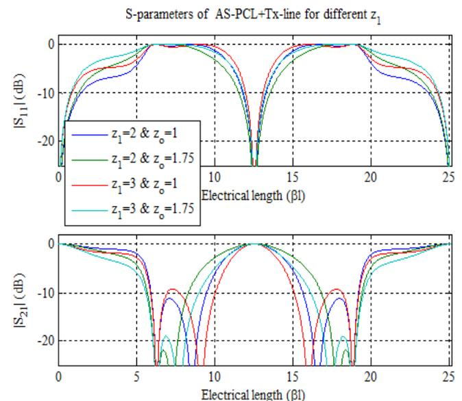
Fig.5 S-parameters of all-stop parallel coupled lines +Tx-line.  $z_c = 2.5$ .
