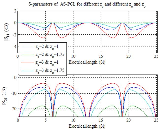
Fig.3 S-parameters of all-stop PCLs with characteristic impedances of 2 and 3 for different even and odd impedances.
