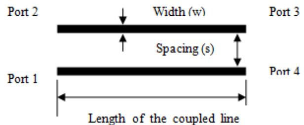
Fig.1 Geometry of the PCL structure.
