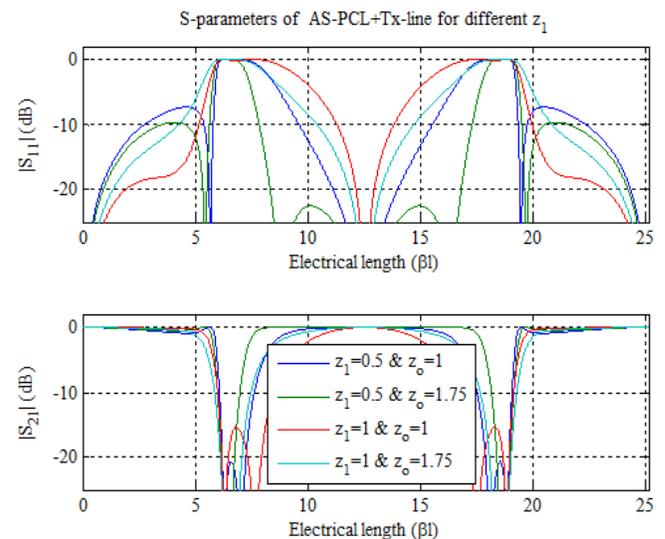
Fig.4 S-parameters of all-stop parallel coupled lines +Tx-line.  $z_c = 2.5$ .
