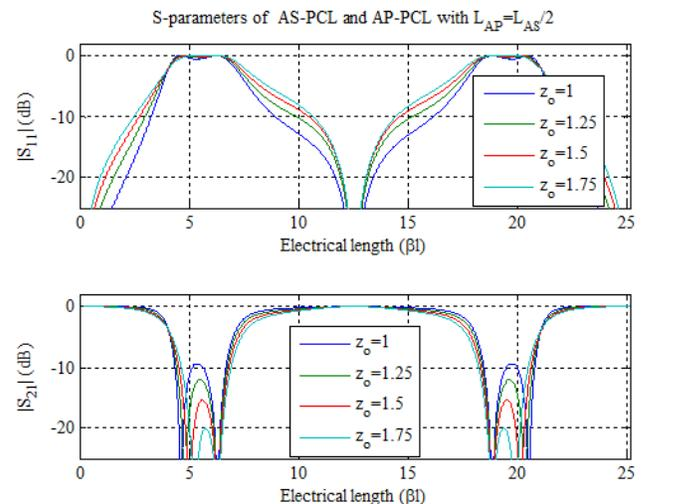
Fig.10 S-parameters of All-stop parallel coupled lines and AP-PCLs (with half length).
