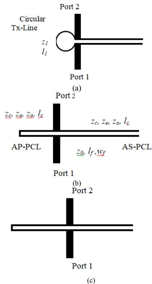
Fig.2 All-pass parallel coupled line with (a) a circular transmission line, (b). all-stop parallel coupled line (half-length), and (c) all-stop parallel coupled line (full length).
