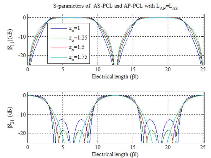
Fig.9 S-parameters of all-stop parallel coupled lines and all-pass PCL with full lengths.
