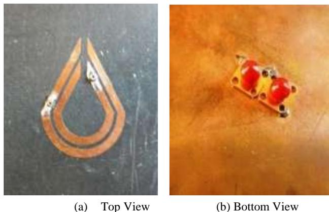
Fig.8. Photograph of the fabricated SSHSS metamaterial antenna
