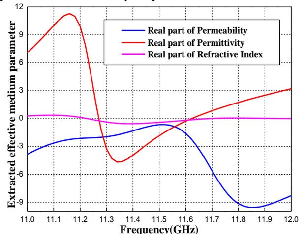
Fig.5. Extracted effective medium parameter from S-parameters
