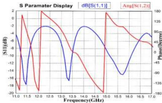
Fig.2.  $S_{11}$  (dB) and  $S_{12}$  (phase angle) of the SSHSS antenna
