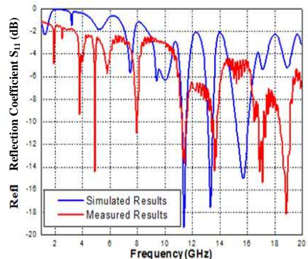
Fig.10. Comparison between simulated and measured reflection coefficient (S<sub>11</sub>)
