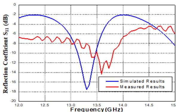
Fig.12. Comparison between simulated and measured reflection coefficient ( $S_{11}$ ) at 13 GHz
