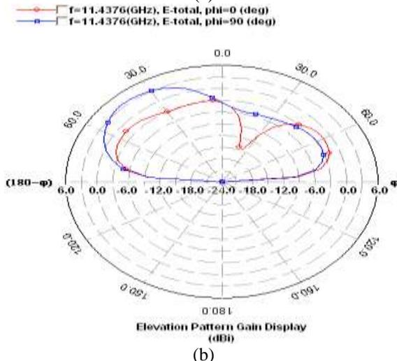
Fig.3. Radiation pattern of the SSHSS antenna (a) azimuth (b) elevation planes
