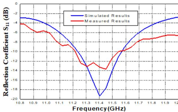
Fig.11. Comparison between simulated and measured reflection coefficient ( $S_{11}$ ) at 11 GHz
