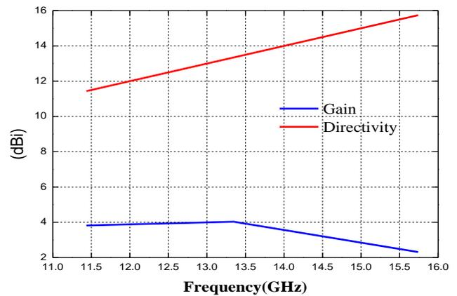
Fig.4. Gain and directivity vs frequency plot of antenna
