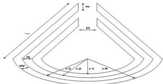
Fig.1. Geometry of split semi-horse shoe structure (SSHSS)
