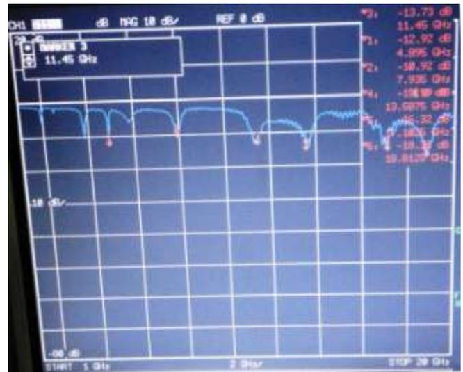
Fig.9. Measured reflection coefficient (S11) of the antenna on VNA
