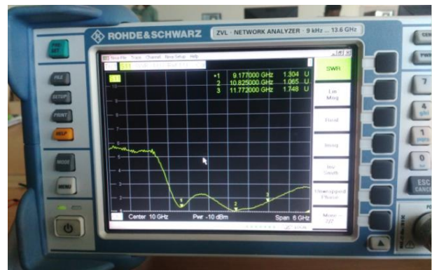
Fig.4. Measured VSWR of the fabricated antenna
