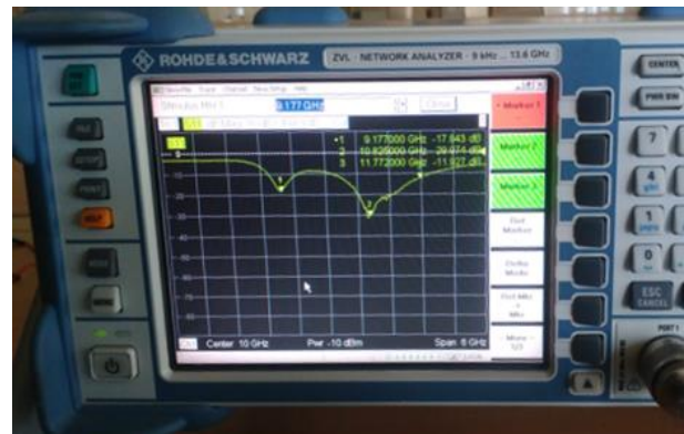
Fig.3. Measured reflection coefficient of the fabricated antenna
