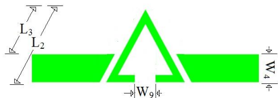
Fig.1. Structure of open loop triangular ring resonator coupled in series with the transmission line.
