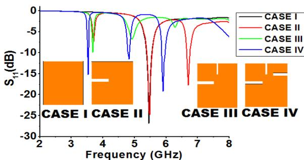
Fig.3.  $S_{11}$  variations of the antenna in different cases
