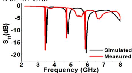
Fig.11. Simulated and measured  $S_{11}$  parameter
