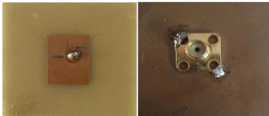
Fig.2. Fabricated structure of the proposed antenna
