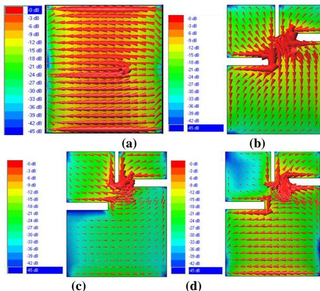
Fig.10. Current distribution of conventional antenna and proposed antenna at (a) 5.5 GHz, (b) 3.51 GHz, (c) 4.82 GHz, (d) 5.90 GHz
