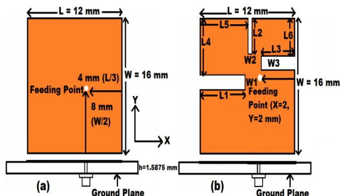
Fig.1. Configuration of (a) Antenna 1 (b) Antenna 2
