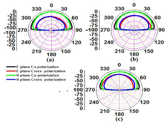
Fig.13. Radiation pattern of proposed antenna (a) 3.51 GHz, (b) 4.82 GHz, (c) 5.90 GHz
