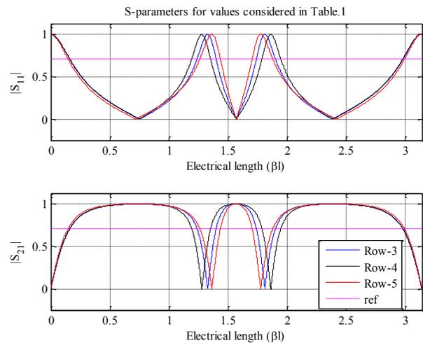
Fig.5 Frequency response of the proposed structure with respect to values considered in Table.1
