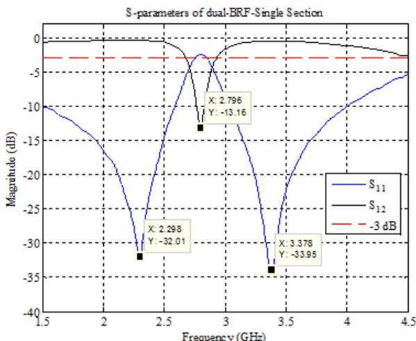
Fig.7 Single section parallel coupled lines structure with short circuits as Row-3 of Table.1.
