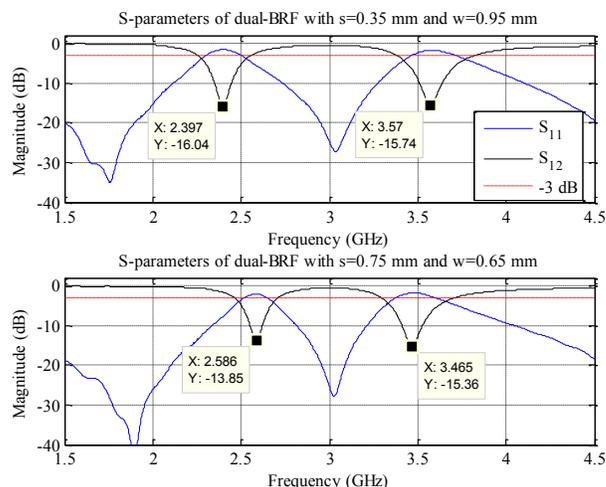
Fig.9 Frequency response of single section dual band reject resonator with different widths and separations.
