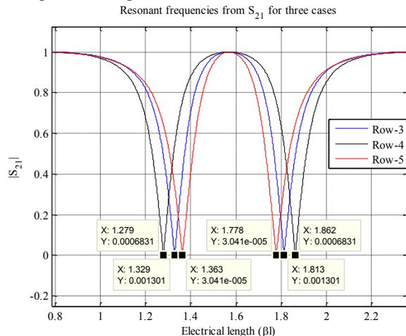
Fig.6 Enlarged view of resonant frequencies for three cases considered in Table.1
