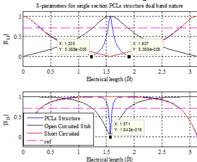
Fig.3 Single section parallel coupled lines structure with short circuits.
