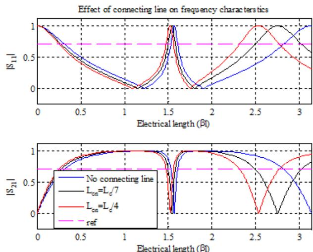
Fig.4 Effect of connecting line on parallel coupled lines structure with short circuits.
