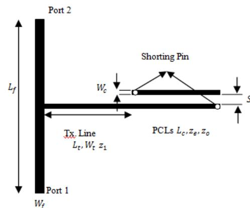
Fig.1 Microstrip layout of the proposed structure.
