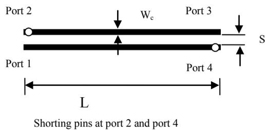
Fig.2 Parallel coupled lines structure with short circuits.
