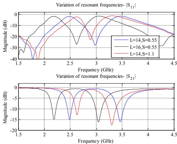
Fig.10 Frequency response of single section dual band reject resonator with different separations and lengths.
