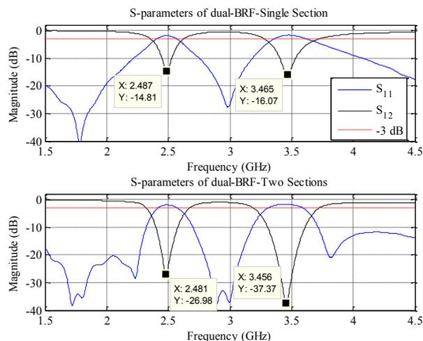
Fig.8 Frequency response of single and cascaded sections of dual-band reject resonator.
