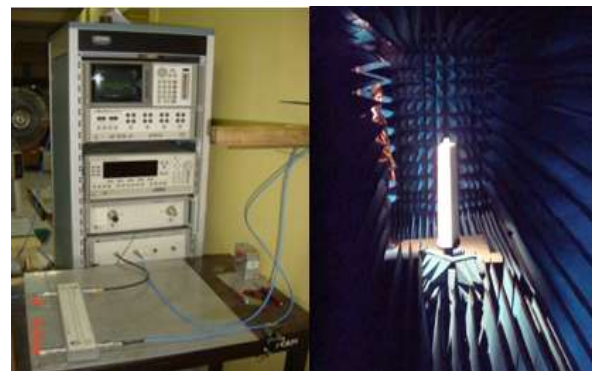
Fig. 6. VNA instrumentation and anechoic chamber for RCS measurements.
