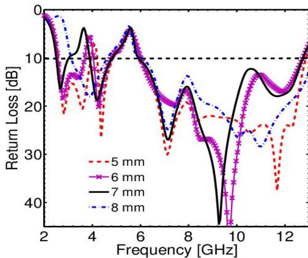
Fig. 7. Effect of the length  $L_s$  of the L-shaped slit on the simulated return loss of the dual band-notch UWB antenna; other parameters are the same as listed in Table 1
