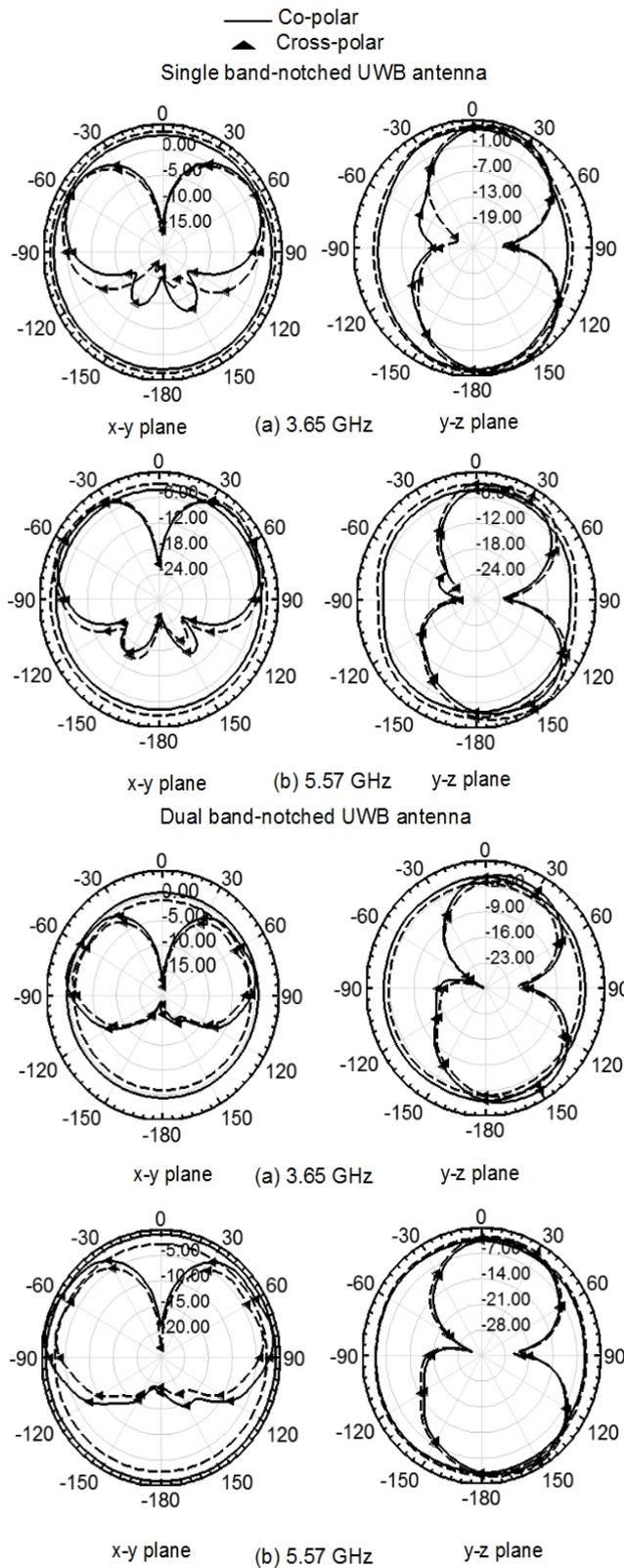
Fig. 10. Radiation pattern for various resonance frequency for the proposed UWB microstrip antenna with single and dual band-notched characteristics — Measured - - - Simulated at (a) 3.65 GHz (b) 5.57 GHz.
