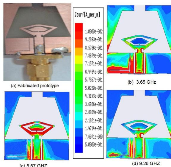
Fig. 6. Dual band-notched Diamond Shaped Monopole UWB antenna (a) Fabricated photograph (b) Current distribution at 3.65 GHz, (c) Current distribution at 5.57 GHz (d) Current distribution at 9.26 GHz.
