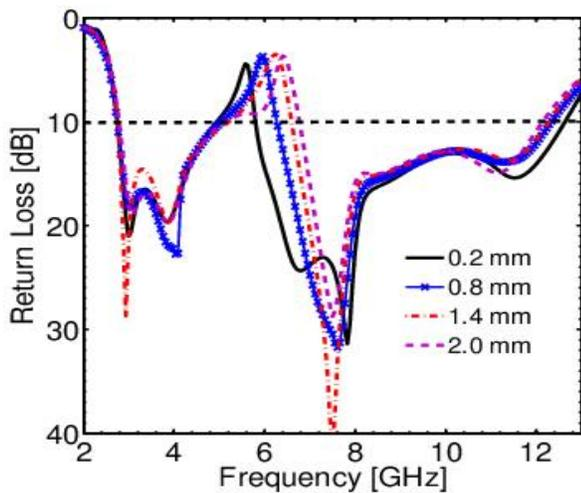
Fig. 3. Effect of  $W_p$  of the C-shaped slit on the simulated return loss of single band-notched UWB antenna; other parameters are the same as listed in Table 1.
