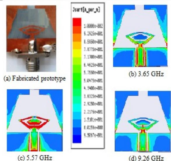
Fig. 2. Single band-notched diamond shaped monopole UWB antenna (a) Fabricated photograph (b) Current distribution at 3.65 GHz, (c) Current distribution at 5.57 GHz (d) Current distribution at 9.26 GHz
