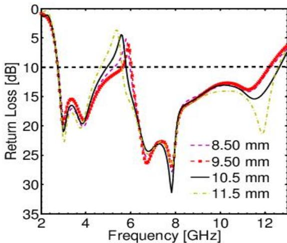
Fig. 4. Effect of the outer width  $W_{p2}$  of the C-shaped slit on the simulated return loss of the single band-notch UWB antenna; other parameters are the same as listed in Table 1
