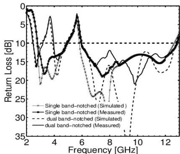
Fig. 9. Simulated and measured return loss of the CPW-Fed Compact diamond Shaped UWB Antenna with single and dual band-notched characteristics
