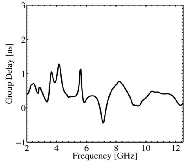
Fig. 12. Group delay of the proposed band-notch diamond shape UWB antenna
